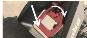
6. Insert the safety pin into the Safety Pin Hole. The safety pin carries no load, but it will prevent the Folding Lever from opening when inserted.
