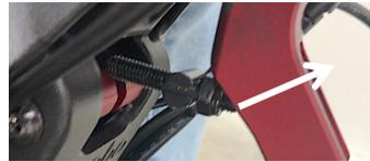
4. Push the front stem forward at the handlebar and pull the Folding Lever upwards so the Folding Shaft moves all the way down into the Slot.
