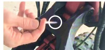
7. Wiggle the front stem to confirm there is no play. If there is play, or the Folding Shaft does not move downwards into its Slot, you need to adjust the position of the Cylinder and Lock Nut on the Folding Shaft. Please have a look at the above referenced video.
