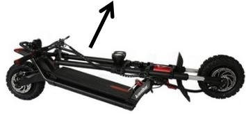
2. Lift up the Folding Lever and push the Folding Shaft downward with your thumb. The other side of the Folding Shaft will move upward.
